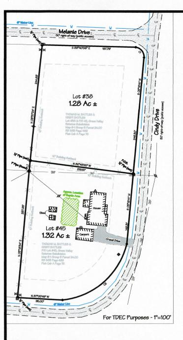
Note: The point of beginning is a  $\frac{1}{2}$ " pipe (set) located in the western right-of-way of Cindy Drive as well as being located N 85°04'36" W 47.45 feet from a power pole and furthermore being located N 10°22'48" E 172.54 feet from a GPS Base Point.
